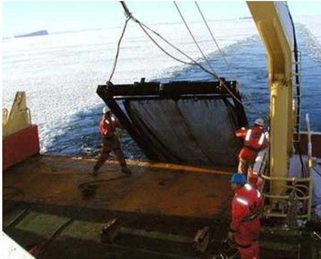
The large white structure at the back end of the vessel on the left is a frame for pulling a large net through the water. On the right a scientific net is being pulled from an ice-covered sea, using the frame at the stern of the ship. This net is put into the ocean and then, using an electronic signal, is opened only when it reaches the depth at which the scientists want to catch fish. Photo courtesy Jose Torres.
